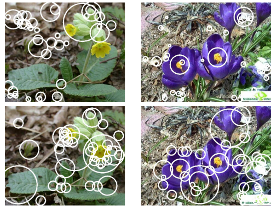
Figure 1: Top row: Laplacian-of-Gaussian and Harris Laplace based on luminance. Bottom row: Laplacian-of-Gaussian and Harris Laplace based on color boosting. The color boosted detector focuses on the more informative features. Only the fifty strongest detected regions are depicted. The radius of the circles indicates the scale selected.
