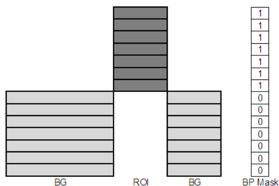
Figure 5.3: MaxShift method, \varphi = 7 . Background is denoted as BG, Region of Interest as ROI and Bitplane mask as BP mask.
