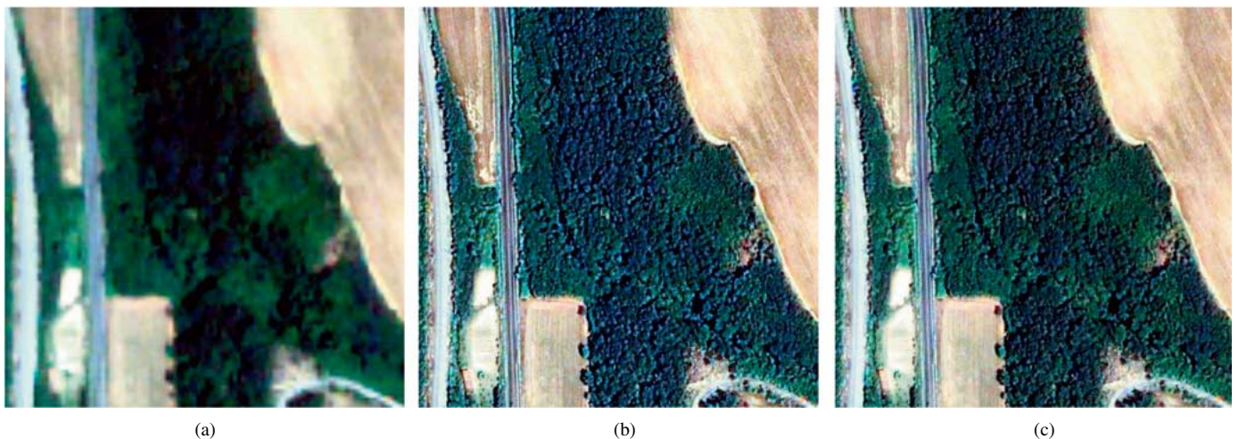
Fig. 5. Color composition ( 400 \text{ rows} \times 400 \text{ columns} ) corresponding to (a) multispectral initial, spatially degraded, image, (b) multispectral AWLP merged image, and (c) multispectral WiSpeR merged image. Images courtesy of Eurimage.
